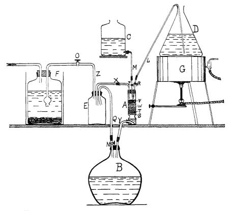
The well-known method of generating gaseous hydrochloric acid by bringing its water solution in contact with strong sulphuric acid was found most convenient. Commercial hydrochloric acid was allowed to flow by gravity from the reservoir C through the
